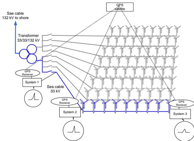
Figure 3 Measuring points at Nysted Offshore Wind Farm
