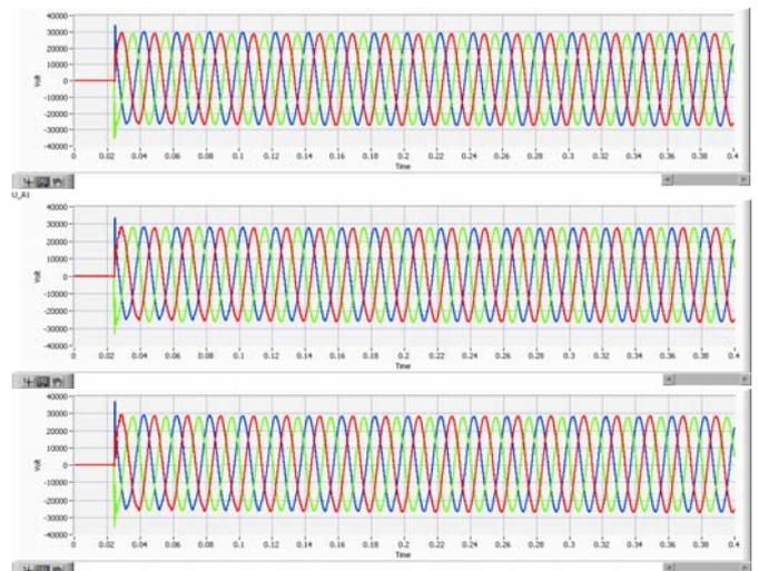
Figure 5 Voltage measurements at three locations during closing of the line breaker. Top: Transform platform, Middle: Turbine A01, Bottom: Turbine A09. Time: 20ms/div
