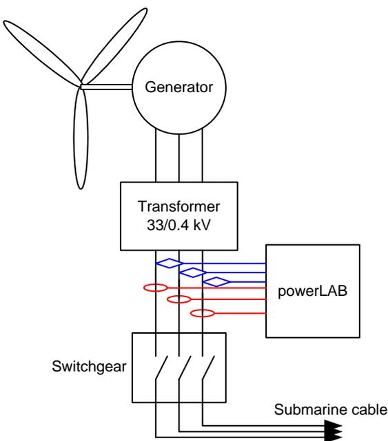
Figure 4 Measuring points in the wind turbine
