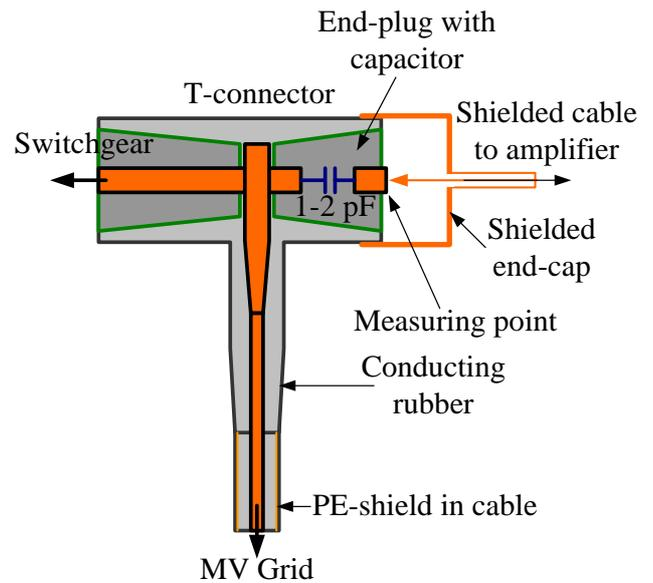
Figure 2 Capacitive measuring end-plug in standard T-connector.
